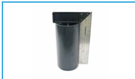
The TP Post must be cut in a straight angle of 90 degrees. Height tolerance between the 4 TP posts per unit is 1 mm.
