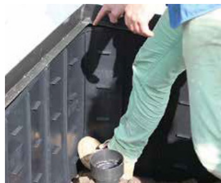
The panels can be folded in a straight angle without breaking.
